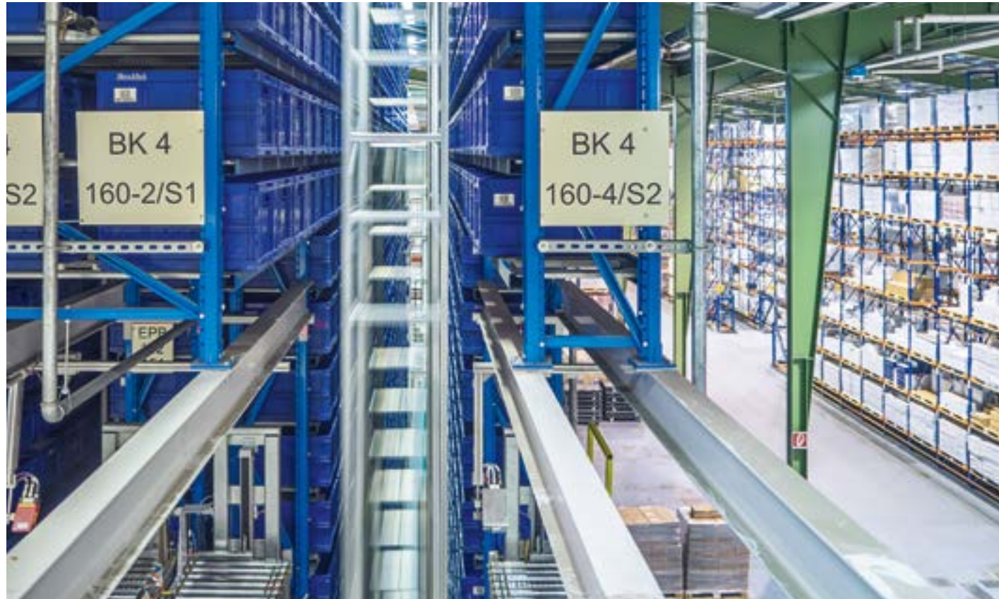
An automated storage and retrieval system removes the containers with the ordered items.
