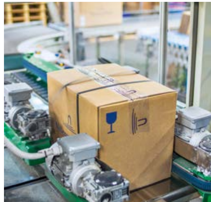
Automatic strapping takes place just before the package is dispatched. On peak days, more than 3,000 packages leave the central warehouse in Merzig.
