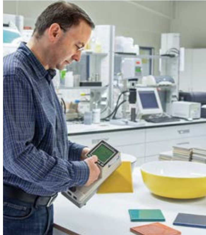
Ceramic engineer Arno Stutz uses a colorimeter to check whether the colour on the product matches the paper sample.
